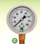
2.5" case diameter, ¼ NPT, bottom connection, stainless steel case and bezel. PC window, brass internals and connection. SSLPG1000 have stainless connector. Grade 'A' Accuracy (1.6%)
