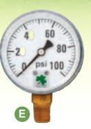
2.5" case diameter, ¼ NPT, bottom connection, stainless steel/ABS case and bezel. PC window, brass internals and connection. Ammonia Gauges have stainless connector. Grade 'A' Accuracy (1.6%)
