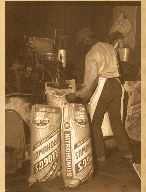
Mill Operator Tommy Mobley and Claudell Carr feed paper sacks through sewing machine before hand-stacking onto flatbed trucks.
